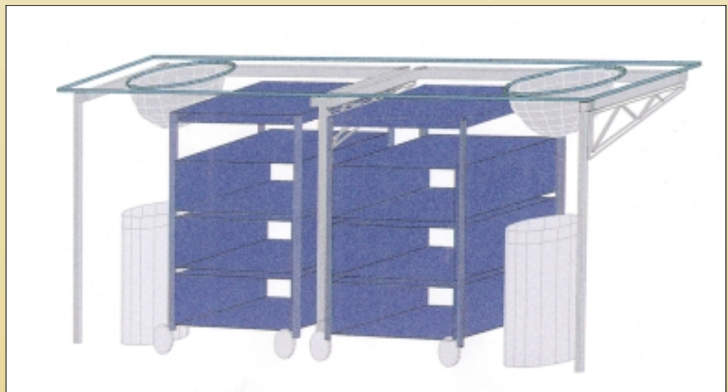
Figure 9: The design for the support structure
