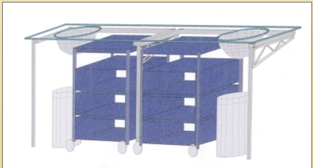
Figure 9: The design for the support structure
