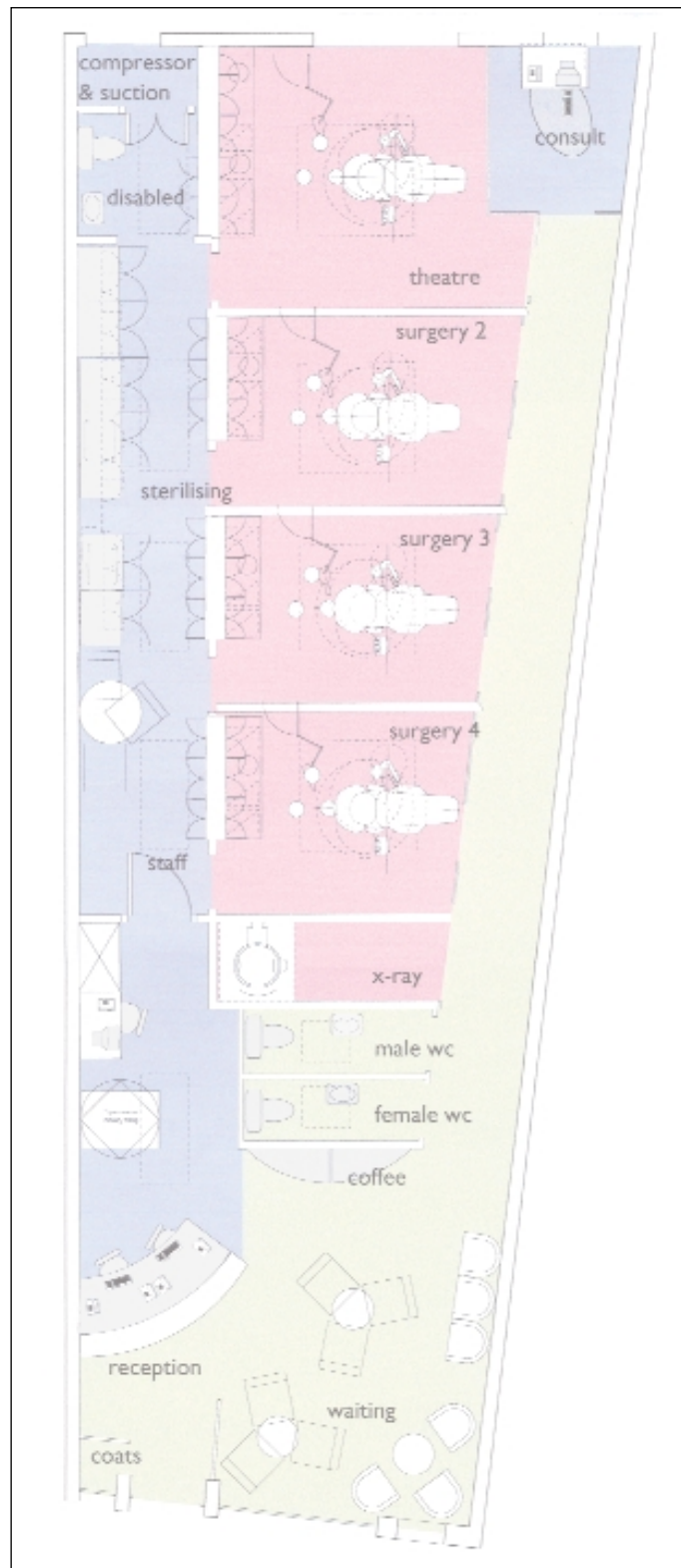
Figure 13: Plan of the practice showing patient access. Corridor (yellow), clinical areas (pink) and staff areas (blue)
