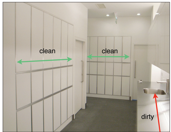
Figures 8 and 9: 'Steri-Walls', a double access, storage wall at the rear of the surgery, can be serviced from the corridor outside and house clean instruments and materials. Separate compartments for waste, services, computer and plugged in sundry appliances. As a separate decontamination area is mandatory, now it is almost as convenient to have a single sided storage wall, replacing conventional dental cabinets. These can be identical to those illustrated but only accessed from the surgery. Figure 9 shows ample clean storage in 'Steri-Walls' accessed from behind the surgery
