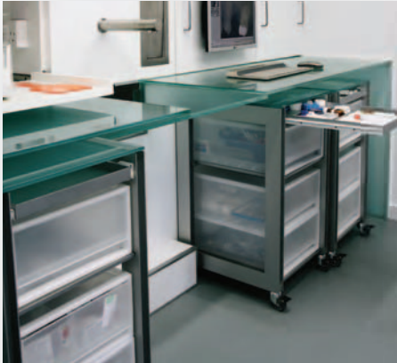
Purpose-made glass-topped trolleys provide further worktop space and feature polypropylene drawers with rounded corners for ease of cleaning
